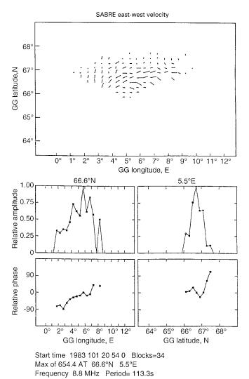
Fig. 7. Amplitude and phase characteristics throughout the SABRE field of view (top) determined from FFT spectral analysis of the SABRE east-west velocity component data on day 101, 1983. The amplitude (middle) and phase (bottom) as a function of latitude are very complicated around the amplitude peak while the longitudinal phase difference of  $\sim 50^{\circ}$  in  $\sim 3^{\circ}$  of longitude implies an m value of  $\sim 17$  and a westward propagating wave
