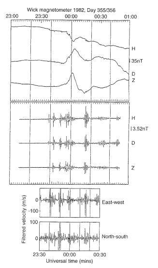
**Fig. 4.** Time series data for the event on day 355/356 1982. From *top to bottom* of the figure, unfiltered and filtered ground magnetometer data from the only operational BGS station at this time (Wick) are presented together with filtered SABRE east-west and north-south velocity component data
