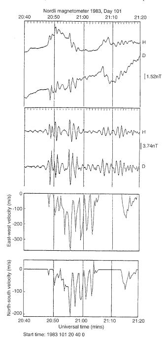
**Fig. 6.** Time series data for the Pi2 pulsations present on day 101, 1983. From *top to bottom*, unfiltered and filtered ground magnetometer data from Nordli are presented together with SABRE east-west and north-south velocity component data. The SABRE data were averaged over the small region of backscatter present during the event, from 66° to 67.6°N and 4° at 6°E
