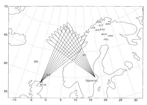
Fig. 1. A schematic diagram to illustrate the location in geographic latitude and longitude of the SABRE field of view, the position of the BGS magnetometers ( $\circ$ ) and the stations of the EISCAT magnetometer cross (+)
