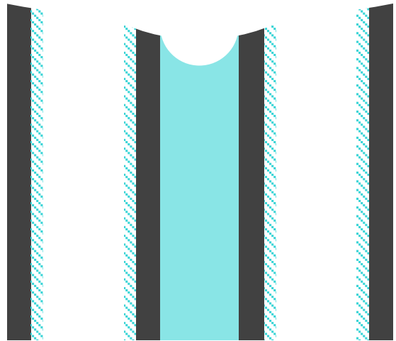
FIG. 6: (Color online). Schematic representation of the deformation of the pore walls (in black) surrounding a filled pore with a concave liquid meniscus. The negative pressure of the liquid in the filled pore contracts its inner walls and reduces the extension of the inner walls of the neighboring empty pores submitted to the spreading pressure exerted by an adsorbed film (hatched zones).
