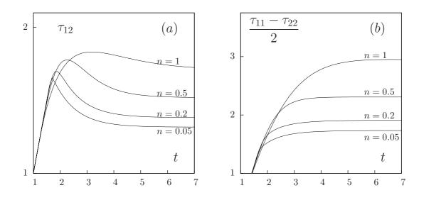
Figure 5: Simple shear flow for a = 1, We = 1, Bi = 1 and  $\alpha = 1$ : (a)  $\tau_{12}$ ; (b)  $(\tau_{11} - \tau_{22})/2$ .
