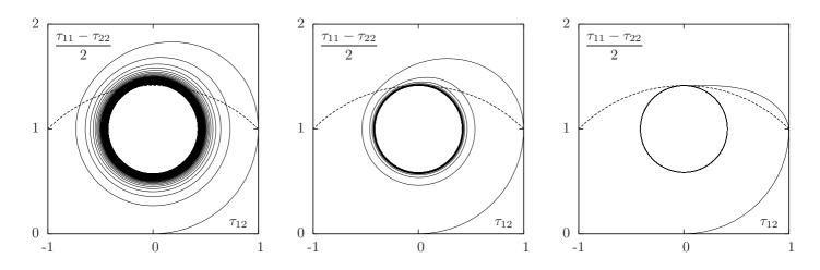
Figure 8: Simple shear flow when a = 0: flow instabilities and asymptotical orbit when (a) n = 0.5; (b) n = 1; (c) n = 2. The dotted line indicates the von Mises circle.
