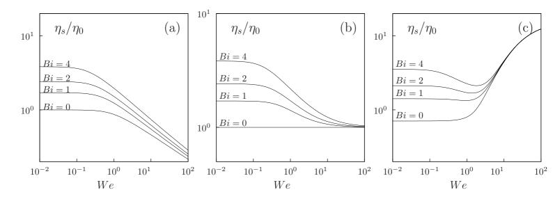
Figure 6: Shear viscosity for a = 1,  $\alpha = 1$  and (a) n = 0.5; (b) n = 1; (c) n = 1.5.
