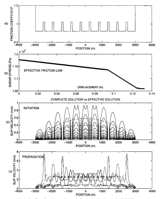
Figure 10. (top) Profile of static resistance along the fault. (middle) Effective friction law used in the computation. (bottom) Comparison between the complete solution (continuous line) and the results obtained with the effective friction law (dashed lines) at the same times. The comparison is presented in the initiation and propagation phases in two separated subplots.
