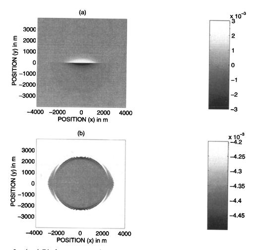
Figure 3. (top) Displacement at a time t = 0.23 s during the initiation as a function of x and y. The computation corresponds to the one presented in Figure 2. (bottom) Derivative of strain with respect to displacement, parameter  $\gamma$ , as a function of x and y at the same time. The value of  $\alpha_c$  associated with the friction law in the infinite fault theory is  $4.36 \times 10^{-3}$  m<sup>-1</sup>.
