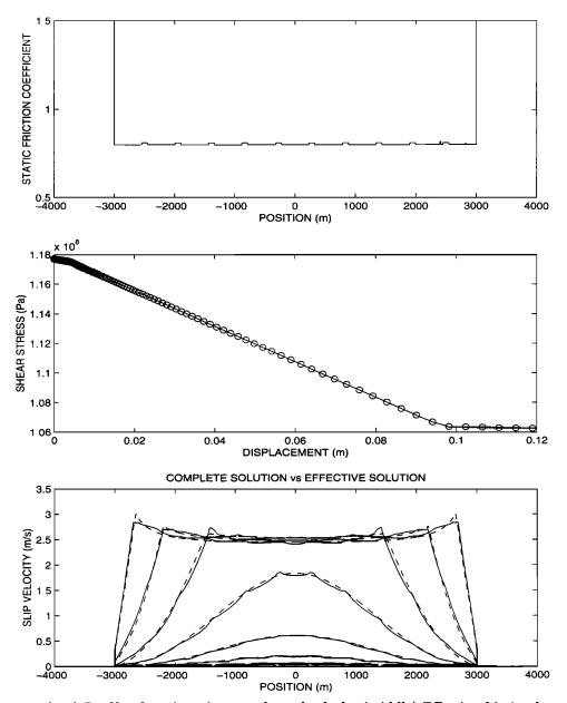
Figure 6. (top) Profile of static resistance along the fault. (middle) Effective friction law used in the computation. (bottom) Comparison between the complete solution (solid line) and the results obtained with the effective friction law (dashed lines) at the same times.
