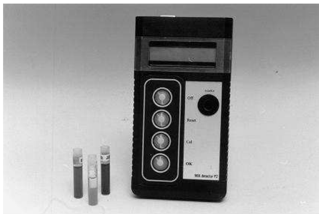
Figure 6. The current magnetic permeability meter, a portable version of the device ( Reprinted from [21] with permission from Elsevier ).
