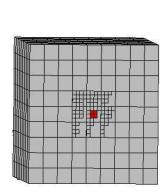
**Figure 6a.** Cube and heterogeneous patch meshes
