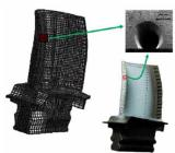
Figure 1. Multiperforated turbine blade
