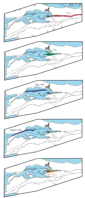
**Figure 8.** The most plausible location of earthquake ruptures between 1719 and 1894, consistent with morphologic observations (Armijo *et al.* 2005), historical data (e.g. Ambraseys & Finkel 1991, 1995) and distribution of slip deficit at any elapsed time. This corresponds to scenarios a and b in Fig. 6, which only differ in the precise location of the 1754 and 1894 events in the Cinarcik basin.
