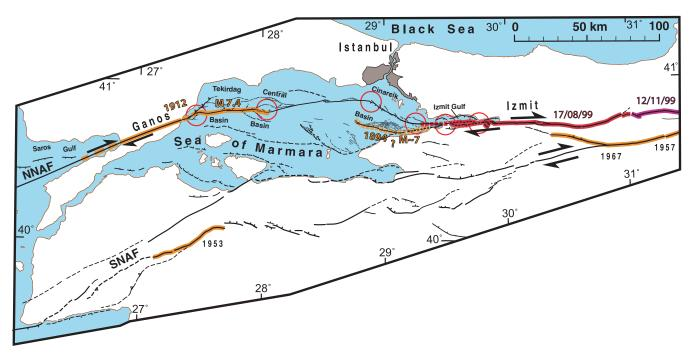
Figure 2. Segmentation of the fault system and recent earthquake ruptures in the Sea of Marmara pull-apart (redrawn from Armijo *et al.* 2002, 2005). The red circles indicate the geometric complexities (jogs and fault-bends) that may be associated with the initiation and termination of  $M \ge 7.0$  earthquake ruptures.
