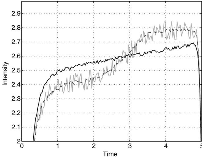
Fig. 7. Experimental data. (Solid gray line) Measured signal versus (solid dark line) standard Kalman filter estimate and (dashed line), proposed filter estimate.
