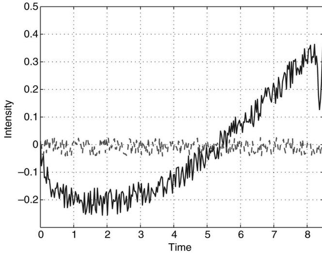
Fig. 6. Benchmark problem. Estimation error for the (solid line) standard Kalman filter and the (dashed line) proposed filter.
