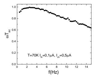
Fig. 2. Frequency dependence of the temperature modulation times the pulsation at 70K. The maximum of this curve (adiabatic plateau) gives the frequency at which the system can be considered as quasi-adiabatic. The alternating current was  $0.5~\mu A$  and the measuring current in the thermometer was  $0.1\mu A$ .
