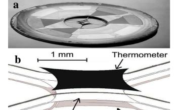
Fig. 1. a-Photograph of the parylen suspended sensor made of a circular copper ring with the electrical contacts and in the center the suspended membrane containing the sensitive part of the sensor. b-Schematic view of the parylen suspended membrane with the thermometer and the ac-heater.
