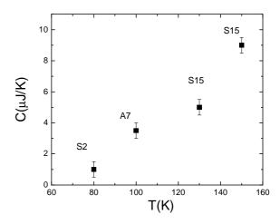
Fig. 3. Measurement of the heat capacity of different sensors at various temperatures between 2Hz and 4Hz. Due to the high fragility of the membrane it has been difficult to vary the temperature on a given sensor. A typical heat capacity of 1microjoule/K is measured at nitrogen temperature.
