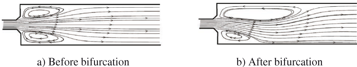
Figure 6. Streamlines before bifurcation for Re = 51 and after bifurcation for Re=68 ( \alpha = 50^\circ , E = 4 and E_d = 2 )
