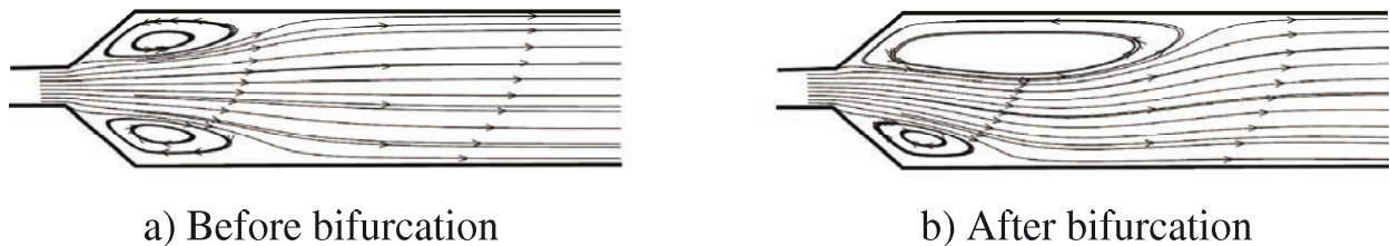
Figure 5. Streamlines before bifurcation for Re = 53 and after bifurcation for Re=90 ( \alpha = 40^\circ , E = E_d = 4 )
