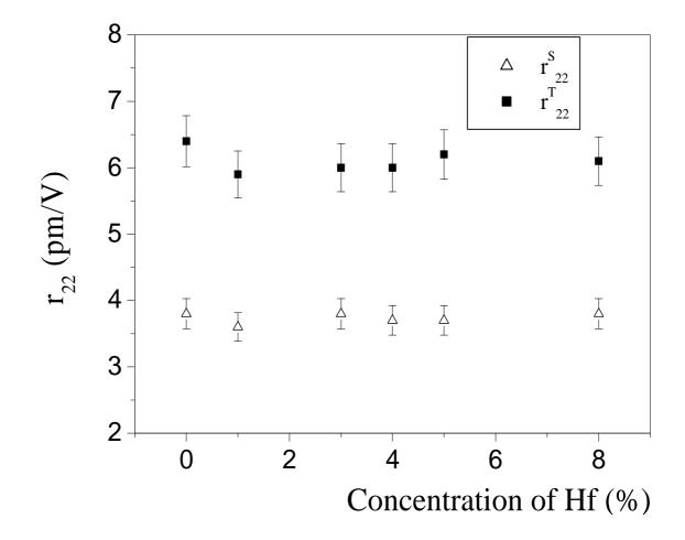
**Fig.4.** EO coefficient  $r_{22}$  versus Hf concentration in congruent LN.
