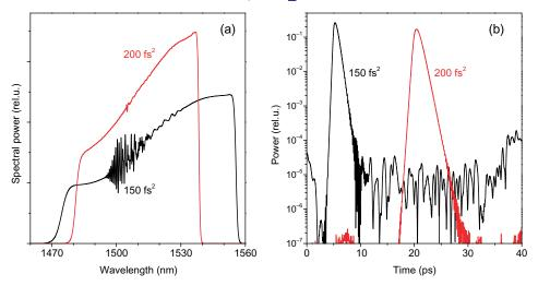
**Figure 7.** (a) Simulated spectra; (b) intensity profiles.  $\beta_2 = 200 \text{ fs}^2$  (red curves) and 150 fs<sup>2</sup> (black curves), respectively. Other parameters correspond to figure 5, the case with spectrally dependent losses.
