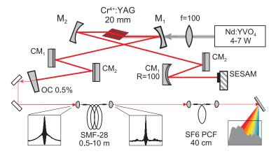
**Figure 1.** Schematic diagram of the Cr:YAG chirped-pulse oscillator. CM: chirped mirrors; OC: output coupler.
