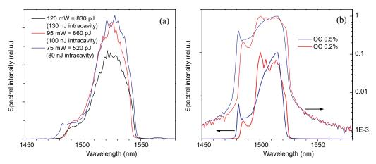
**Figure 3.** (a) Spectra of the Cr : YAG CPO at different values of intracavity pulse energy. (b) Spectra of the Cr : YAG CPO with different output couplers.
