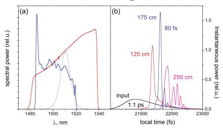
**Figure 5.** (a) Spectral profiles: GDD at  $\lambda'_0$  is 200 fs<sup>2</sup> (red and blue curves) and  $-9900 \text{ fs}^2$  (gray curve). For the blue curve, the spectral losses are not taken into account. (b) Pulse profiles inside a fiber for the input pulse corresponding to the red solid curve in (a). Propagation lengths are indicated; minimum pulse width  $\approx 80 \text{ fs}$ .
