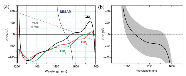
**Figure 2.** (a) GDD of three sets of chirped mirrors (as designed), the YAG crystal, and the SESAM. (b) The net dispersion of the resonator, corresponding to figure 1. Black line: as designed, gray area—uncertainty region due to the chirped mirrors.
