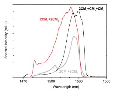
**Figure 8.** Experimental spectra of the CPO regime. The intracavity dispersion is changed by exchanging the mirrors. The actual mirror sets are used as labels. Red  $(2CM_1 + 2CM_2)$  and black  $(2CM_1 + CM_2 + CM_3)$  curves correspond to the CPO regime; the gray curve  $(2CM_1 + 2CM_3)$ , not to the scale) represents a 'chaotic' mode-locking regime. Exchange of one CM<sub>2</sub> mirror by a CM<sub>3</sub> mirror reduces the round-trip GDD by about -40 fs<sup>2</sup> at 1.53  $\mu$ m.
