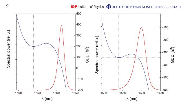
**Figure 6.** GDD spectral profiles (blue) and corresponding simulated pulse spectra (red) with no spectral dependence of the losses.
