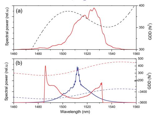
**Figure 9.** Simulated spectra (solid curves), with different net GDD values (dashed curves).  $\lambda_0 = 1.54 \,\mu\text{m}$ ; other parameters correspond to figure 5, the case without spectrally dependent losses.
