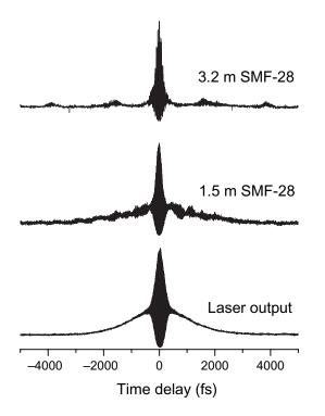
Figure 4. Extra-cavity pulse compression by a single-mode silica fiber.
