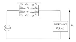
Fig. 3: Vdd-hopping, voltage supply and load
