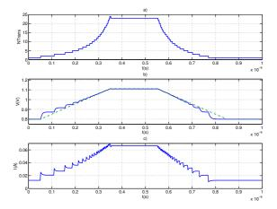
Fig. 7: Control No. 3. a) Evolution of the number of switchedon PMOS, b) evolution of the  $v_r$  (dashed) and evolution of  $v_c$ (solid). c) evolution of the current  $I_l$ .
