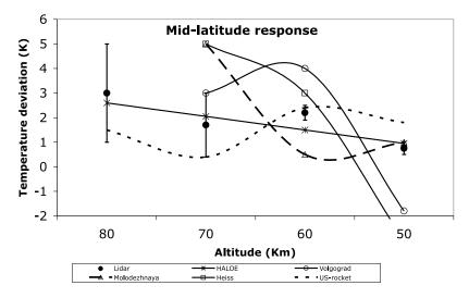
**Figure 3.** Atmospheric temperature response to the 11-year solar cycle as a function of altitude from different studies covering midlatitudes. Error bars associated with the OHP lidar correspond to the range of seasonal changes [*Keckhut et al.*, 2005]. US-rocket corresponds to an average of three subtropical rocket stations [*Keckhut et al.*, 1999]. The Russian rocket sites (Volgograd, Molodezhnaya, and Heiss) have been analyzed by *Kokin et al.* [1990] and *Golitsyn et al.* [2006].
