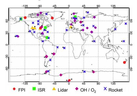
**Figure 1.** Ground-based mesospheric and lower thermospheric data stations for the measurements of temperature. FPI represents Fabry-Perot interferometer, and ISR represents incoherent scatter radar. Those stations whose results have been used in the present paper are marked with asterisks.
