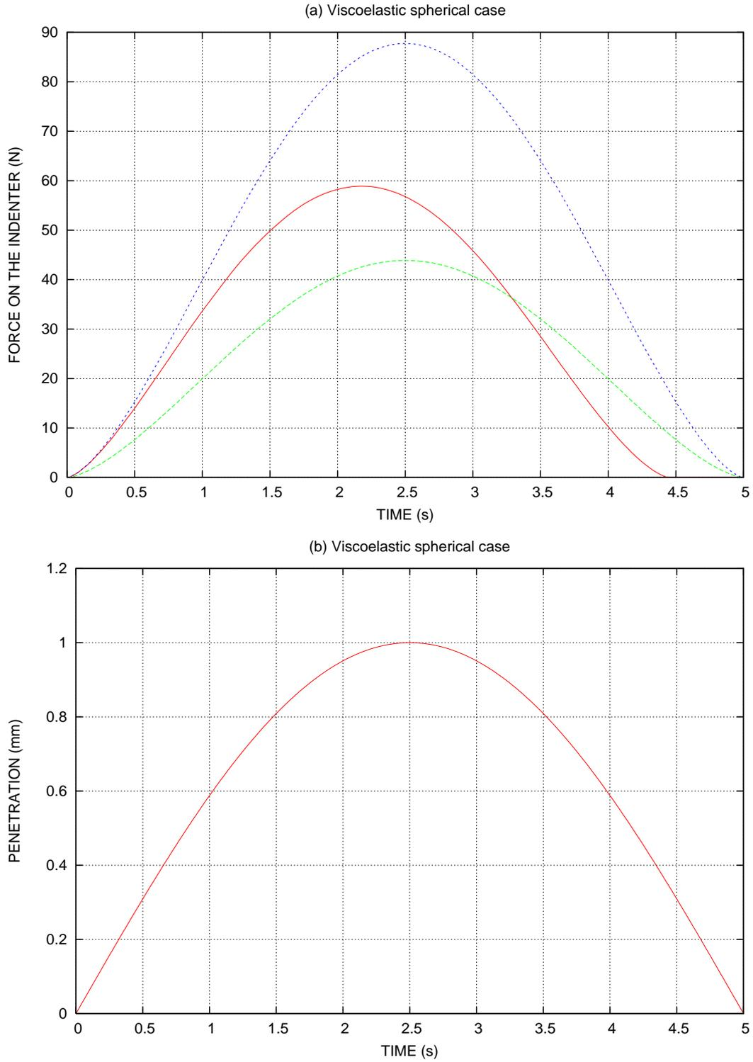
Fig. 6. Spherical case. The penetration  $\delta(t)$  is imposed (a) The difference between the contact forces, — viscoelastic numerical, - - - - elastic with  $E_\infty = 7.5$  MPa, ..... elastic with  $E_0 = 15$  MPa (b) The penetration  $\delta(t)$
