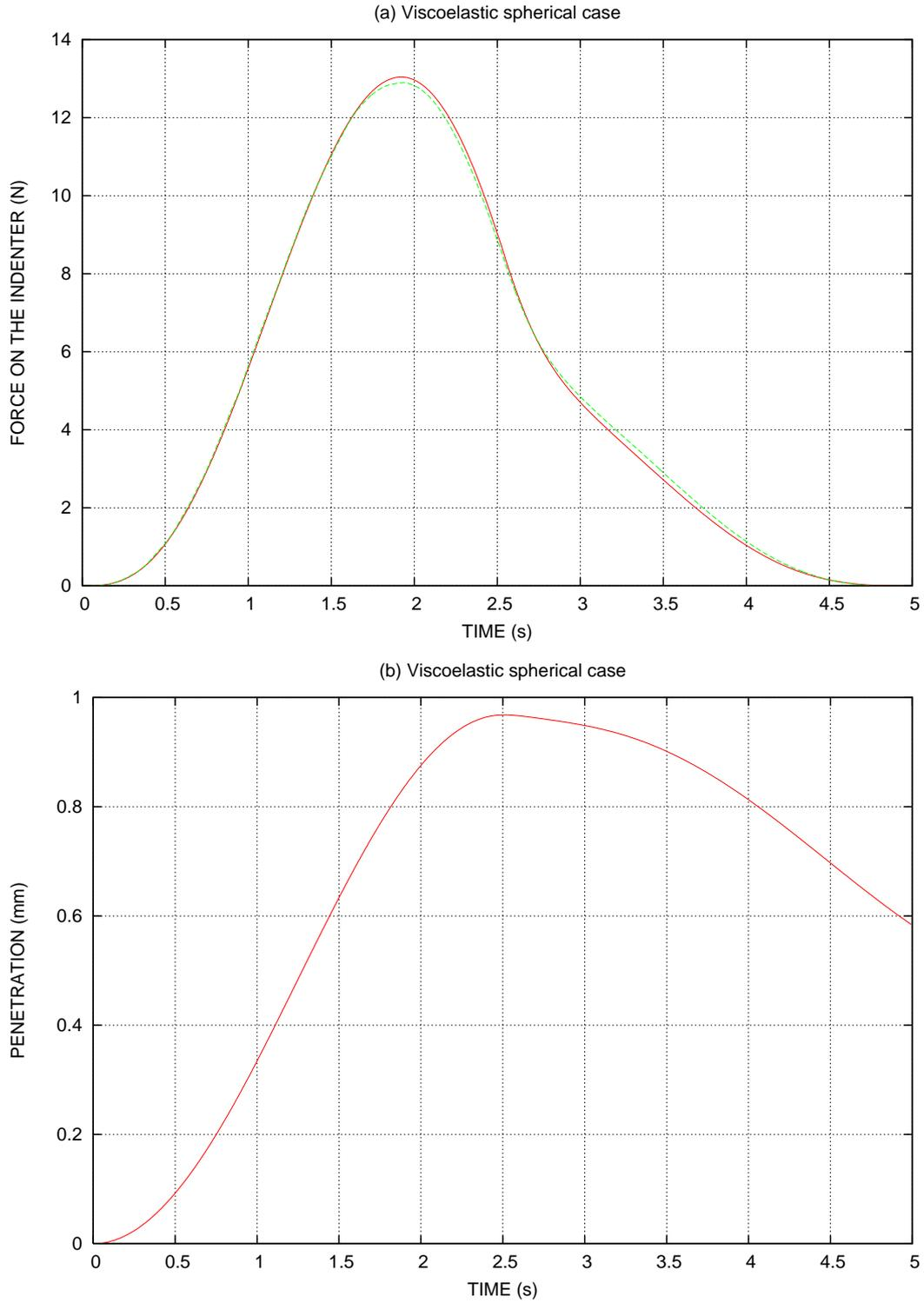
Fig. 5. Spherical case. The contact radius  $a(t)$  is imposed. Strongly time dependent material (a) The difference between the contact forces, — viscoelastic analytical, ---- viscoelastic numerical (b) The penetration  $\delta(t)$
