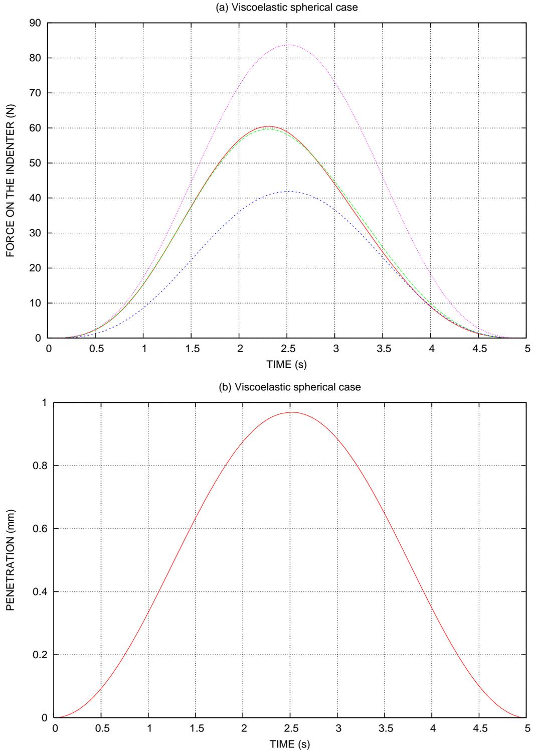
Fig. 4. Spherical case. The contact radius  $a(t)$  is imposed (a) The difference between the contact forces, — viscoelastic analytical, ----- viscoelastic numerical, ..... elastic with  $E_\infty = 7.5$  MPa, ..... elastic with  $E_0 = 15$  MPa (b) The penetration  $\delta(t)$
