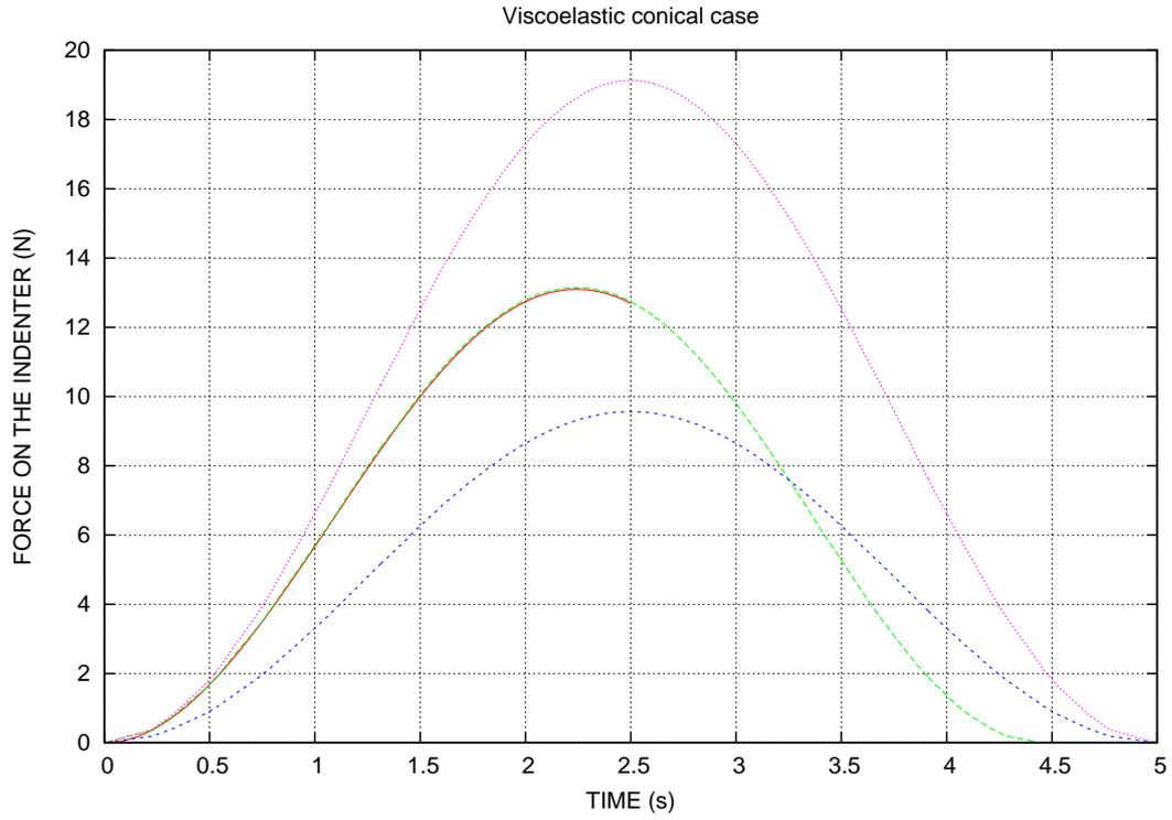
Fig. 10. Conical case. The penetration  $\delta(t)$  is imposed. The difference between the contact forces, — viscoelastic analytical, ----- viscoelastic numerical, ..... elastic with  $E_\infty = 7.5$  MPa, -·-·-· elastic with  $E_0 = 15$  MPa
