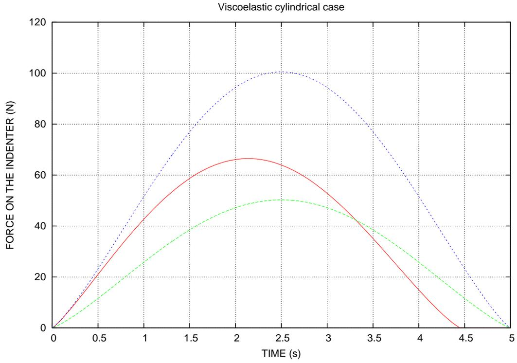
Fig. 14. Cylindrical case. The penetration  $\delta(t)$  is imposed. The difference between the contact forces, — viscoelastic numerical, - - - - - elastic with  $E_\infty = 7.5$  MPa, ····· elastic with  $E_0 = 15$  MPa
