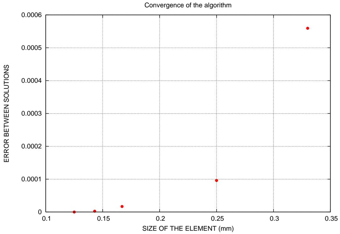
Fig. 9. Spherical case. Convergence of the algorithm
