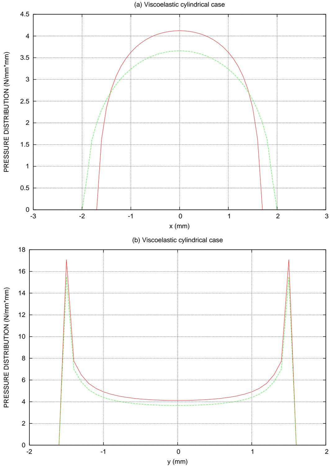
Fig. 13. Cylindrical case. The pressure distribution for  $t_1 = 1.25$  s and  $t_2 = 3.05$  s (a)  $y = 0$  mm, — viscoelastic for  $t_1$ , - - - viscoelastic for  $t_2$  (b)  $x = 0$  mm, — viscoelastic for  $t_1$ , - - - viscoelastic for  $t_2$
