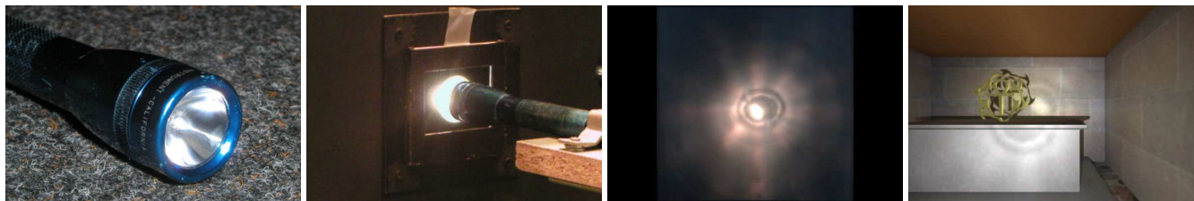
Figure 1: Stages of light source measurement and rendering (from left to right): a) photo of flashlight – b) flashlight in measurement setup – c) 2D reconstruction of the measured data in a virtual plane – d) measured light used in a global illumination simulation.
