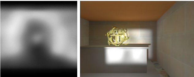
Figure 10: Mag-Lite acquisition with Setup A: Left, a projection on a distant (3 m) plane, Right: a global illumination solution (Importance table construction - 20 s, Particle emission - 40 s, Rendering 20 min). The acquired data set was converted to grayscale.
