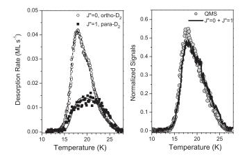
FIG. 3. D<sub>2</sub> desorption after deposition of 1.5 ML of D<sub>2</sub> on 10 ML porous ASW ice at 10 K. Right side; filled gray circles: QMS signal, dotted line: normalized sum with coefficient (see text) of the J'' = 0 and J'' = 1 desorption. Left side; circles J'' = 0 desorption signal; full squares: J'' = 1 desorption signal, solid lines: modeling.
