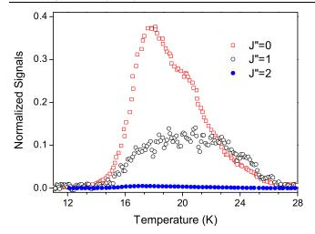
FIG. 2 (color online). D<sub>2</sub> desorption after deposition of 1.5 ML of D<sub>2</sub> on 10 ML porous ASW ice at 10 K. Square: J'' = 0 rotational state (average of 5 measurements); empty circles: J'' = 1 rotational state, full circles: J'' = 2 rotational state (average of 3 measurements). The data have been averaged with 20 points (each point in the figure represents 1 s).
