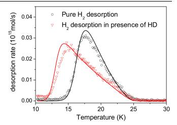
FIG. 1 (color online).  $H_2$  Desorption after deposition of 0.7 ML (1 ML =  $1 \times 10^{15} \text{ mol/cm}^2$ ) on 10 ML porous ASW ice at 10 K. Desorption without any other adsorbate (circles), and in presence of 0.5 ML of HD (triangles). Solid lines: result of our model fitting simultaneously several isotopic mixtures at various doses.
