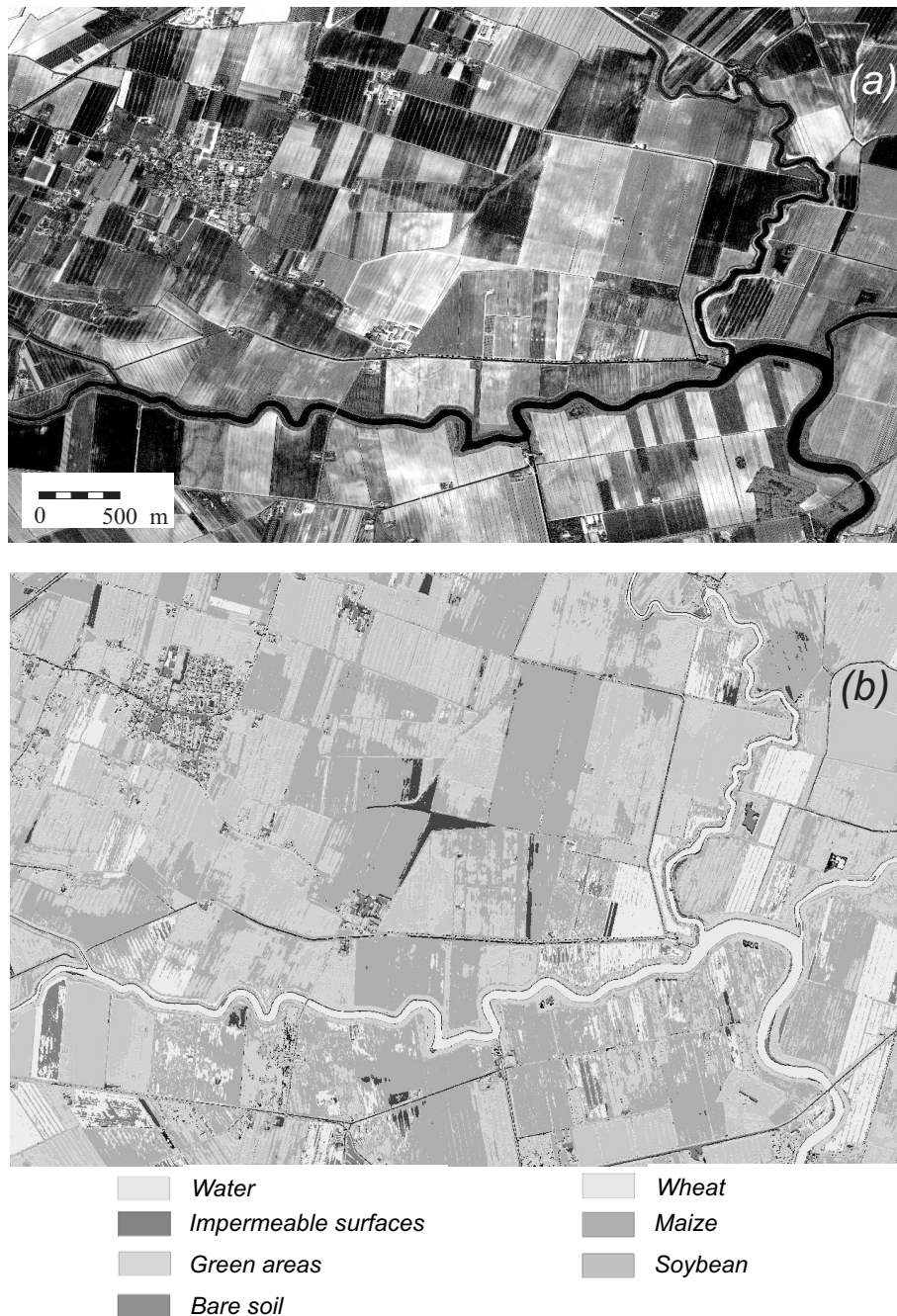
Fig. 3. Remote sensing tools: example of land-use classification of a small area in the test catchment between the outlet and the Venice Lagoon. The classification procedure is applied to the entire basin and employs characteristic ratios of relevant soil parameters coarse grained at the scale of source areas. Fraction of agricultural areas are used to estimate total nitrate mass in immobile phases. Technical details can be found in Rinaldo et al. (2003).
