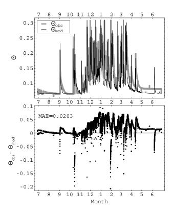
**Fig. 10.** Observed and modelled half-hourly surface soil moisture  $(\theta_{obs} \text{ and } \theta_{mod} \text{ respectively, m}^3 \text{ m}^{-3})$  (top) and their residuals (bottom) obtained using a fixed root distribution. MAE denotes the mean absolute error of the model.
