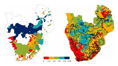
**Fig. 11.** Baseflow indices at discharge observation stations in Southern Africa, mapped onto the pertaining basins (Bullock et al., 1997, their Fig. 4.35) (left); groundwater recharge as a fraction of total runoff from land as computed with WGHM, with polygon outlines of Bullock et al. (1997) for easier comparison (right). Please note that the polygon outlines are not basin boundaries but boundaries of polygon with the same color in the figure on the left.
