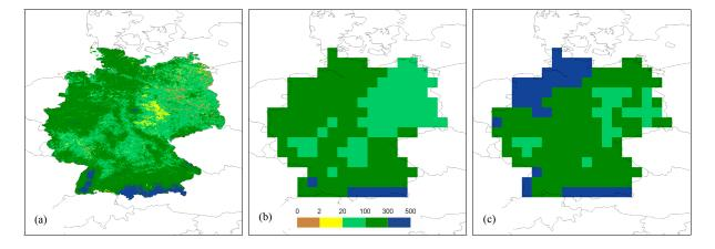
**Fig. 10.** Groundwater recharge in Germany, in mm/yr, as computed by Jankiewicz et al. (2005, their Fig. 9) with a spatial resolution of 1 km by 1 km for 1961–1990 (**a**); aggregated to a spatial resolution of  $0.5^{\circ}$  (**b**); groundwater recharge as computed with WGHM for the same spatial resolution and time period (**c**).
