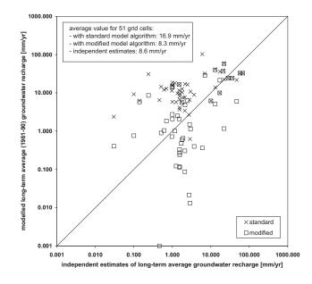
**Fig. 3.** Improved modeling of groundwater recharge due to modified groundwater recharge algorithm for semi-arid regions: comparison of independent estimates of long-term average groundwater recharge for 51 grid cells in semi-arid regions with modeled values as computed with the standard and the modified algorithm (using GPCC precipitation).
