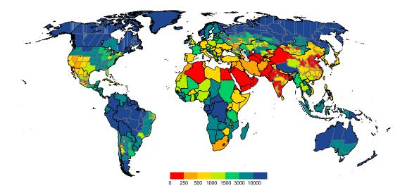
**Fig. 6.** Per-capita groundwater resources in administrative units, in  $m^3/(\text{capita}\,\text{yr})$ , as computed by WGHM (ensemble mean using GPCC/CRU precipitation). Groundwater resources are representative for the climate normal 1961–1990, population is representative for the year 2000.
