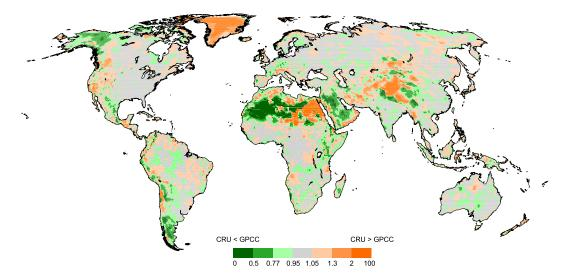
**Fig. 4.** Difference between the two available 0.5° global data sets of time series of gridded observed precipitation: ratio of CRU 1961-1990 mean annual precipitation to GPCC 1961-1990 mean annual precipitation.
