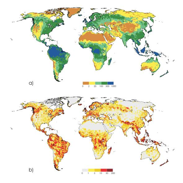
**Fig. 5.** Long-term average diffuse groundwater recharge for the time period 1961–1990 in mm/yr; ensemble mean of groundwater recharge as computed by two WGHM model runs with either GPCC or CRU precipitation data as input (**a**). Absolute difference between groundwater recharge computed with either one of the two precipitation data sets and the ensemble mean value, in mm/yr (**b**).
