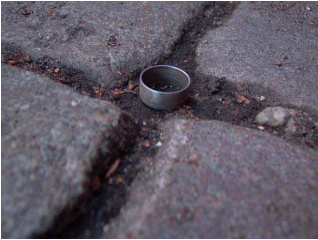
Fig. 3. Undisturbed sampling of seam material (0 to 1 cm) from a cobblestone paved street using special 3.3 cm 3 cylinders in an old residential area at the site Pfluegerstrasse, Berlin.
