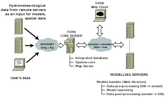
Fig. 2. Communication between core system and surrounding subsystems.
