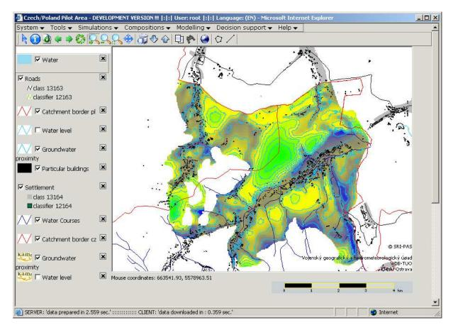
Fig. 4. Groundwater level (both isolines and raster) as a result of ModFlow model presented by web client.
