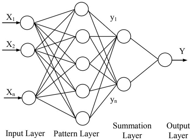
Fig. 4. The general structure of a GRNN.
