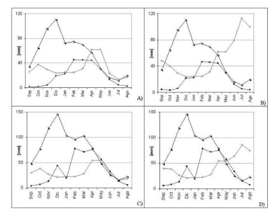
**Fig. 6.** Water budget calculation [mm/month] for the case of land exploitation (right) and for current land use (left) for the Flumini (above) and Mogoro (below) basins. While precipitation is unchanged, evapotranspiration (line with empty points) and streamflow (line with full points) are affected by the new management practices.
