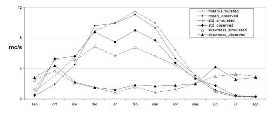
Fig. 5. Comparison of measured and simulated monthly streamflow statistics (mean, standard deviation, and skewness) for the 70-year regional calibration.
