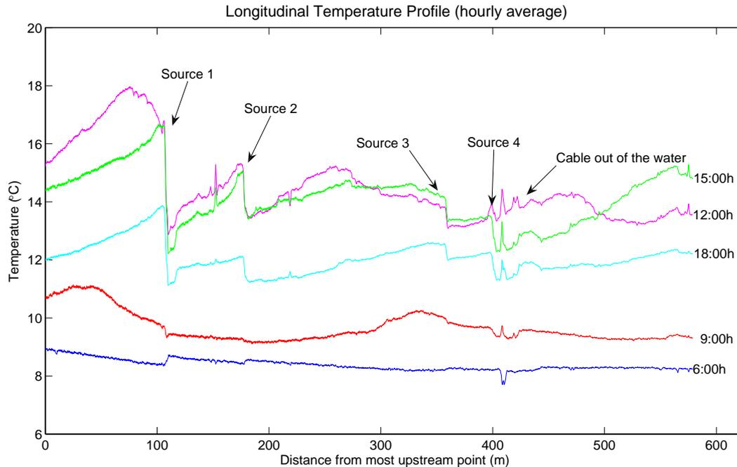
**Fig. 3.** Observed longitudinal temperature profile of the stream at different times at 26 April 2006. Clear temperature jumps can be seen at the points of a source. Short peaks are due to the fact that the cable is out of the water for a short distance.
