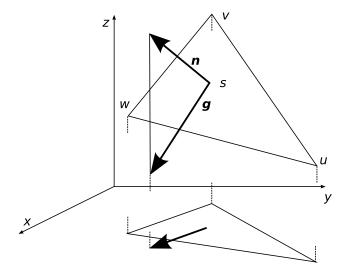
**Fig. 1.** Derivation of the slope gradient for a single triangle. The horizontal projection of the triangle is added to the sketch for illustration.
