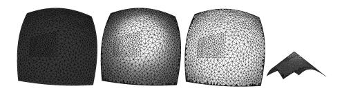
Fig. 6. Water flow on the same triangulated irregular mesh as use for the previous simulations, but now stretched over a cone. The first three images show the soil moisture (white = dry, black = wet) at the beginning and after 10 and 20 time steps, respectively. The cone is observed from the top. The most right image is a side view of the cone.
