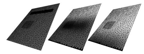
Fig. 4. Water flow on a triangulated irregular mesh describing an inclined plane. The three images show the soil moisture (white = dry, black = wet) at the beginning and after 20 and 40 time steps, respectively.
