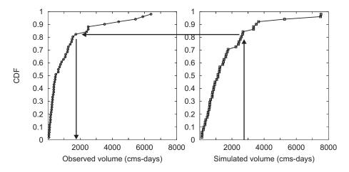
**Fig. 4.** Illustration of the quantile mapping method. The panels show the empirical cumulative distribution function for the observed and simulated monthly flow volume from the historical simulation. The arrows illustrate the transformation of an ensemble trace to the biascorrected ensemble trace.
