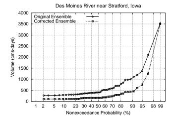
**Fig. 2.** Probability distribution forecasts from Des Moines River ensemble streamflow prediction system for September 1965, with and without bias correction applied to the ensemble traces. The effect of bias correction is to shift the probability distribution forecasts.
