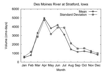
**Fig. 1.** Historical variations in monthly streamflow for the Des Moines River at Stratford, Iowa (USGS 05481300). The plot shows the mean and standard deviation of monthly flow volume (cmsdays) based on the stream-gage record from 1949 through 1996.
