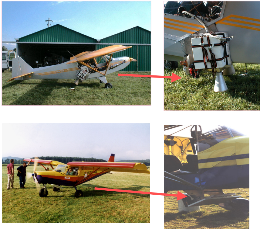
Fig. 1. The installation of the IROE sensors onboard the two ultra- light airplanes: showing the C-band radiometer (top) and the flat microstrip antenna of L-band radiometer (bottom).
