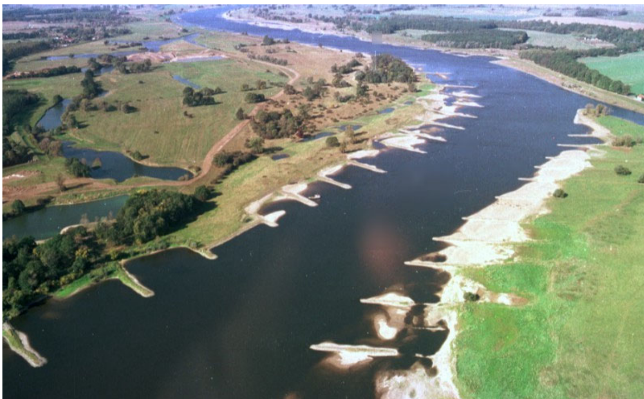
Fig. 2. Aerial photograph of the middle part of the River Elbe with characteristic groyne fields.
