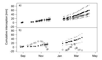
**Fig. 6.** Cumulative totals of calculated (open circles) and estimated (solid circles) interception for maximum 10 min rainfall intensities (a)  $I_{10}$  max $\leq$ 30 mm h<sup>-1</sup> and (b)  $I_{10}$  max>30 mm h<sup>-1</sup> including all collectors (n=20). The dots indicate the uncertainty of the modeled interception resulting from the uncertainty in  $S_C$ .
