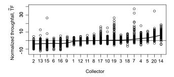
**Fig. 2.** Plot of normalized throughfall,  $\tilde{T}$ , for the whole period. Each circle represents the event throughfall volume at a single collector, normalized to zero median and unit variance for that event. The collectors are plotted on the horizontal axis and ranked by their means,  $\tilde{T}$ , which are connected by the black curve.
