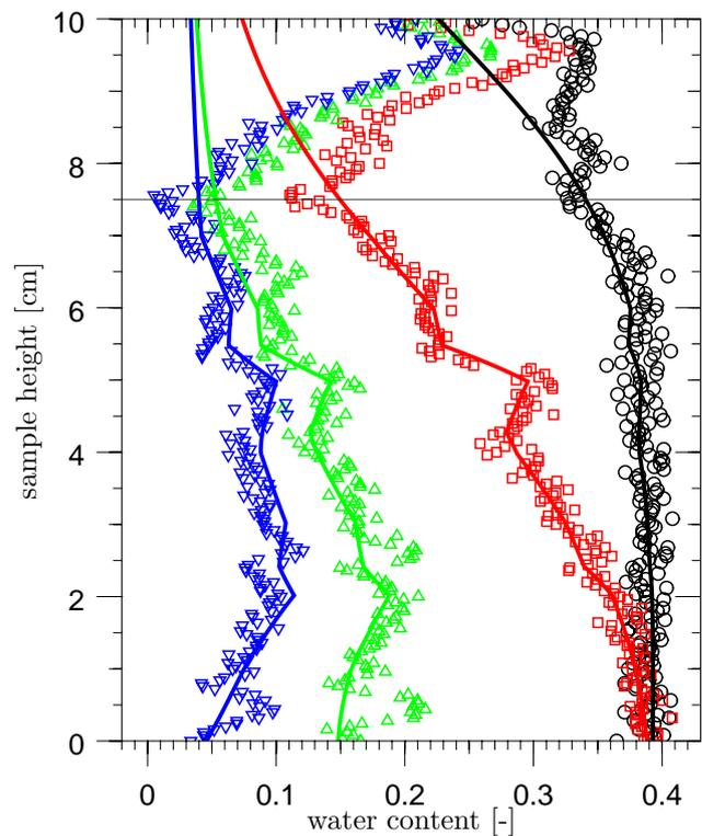
**Fig. 5.** Measured (symbols) and simulated (solid lines) vertical water content profiles assuming a layered sample. The matric head at the lower boundary was  $-8$  cm (black),  $-12$  cm (red),  $-16$  cm (green) and  $-20$  cm (blue) for the shown profiles. Above the horizontal line ( $z=7.5$  cm) the measurements are affected by changes near the sample surface that leads to unrealistic water content values.
