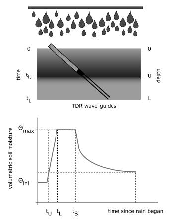
**Fig. 2.** Schematic representation of an obliquely installed waveguide, a downwards travelling wetting front (up) and the linear increase of  $\theta$  as the wetting front moves steadily (below).  $t_S$  indicates end of sprinkling.
