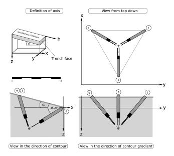
**Fig. 3.** Definition of axis (top left) and scheme of mounting a triplet of TDR wave-guides in a hillslope soil by its different views. Probes (black) are attached to aluminium pipes (dark grey). Note that y-axis becomes positive towards right and negative towards left. And z-axis becomes more positive with increasing depth.
