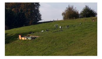
Fig. 1. The Lutertal study site on a grassland slope in northern Switzerland. Note the brownish trench face which was excavated at the bottom end of the instrumented  $100 \text{ m}^2$  plot.
