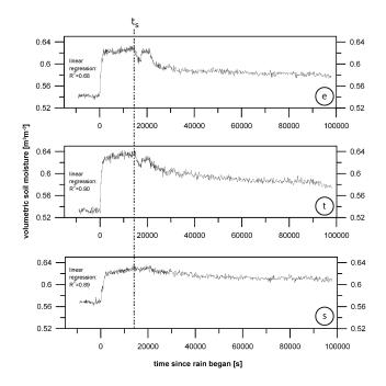
**Fig. 5.** Time-series of volumetric soil moisture for the three TDR wave-guides *e*, *t*, and *s* of triplet E in 11 cm depth on 27/05/2005 (ID #15). A continual, linear increase of soil moisture between  $\theta_{ini}$  and  $\theta_{max}$  is assumed. The analysed coefficients of determination for these slopes are mentioned next to the graphs.
