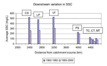
Fig. 8. Sediment concentration variation along the Lower Mekong.
