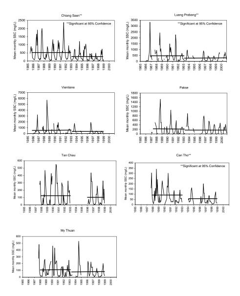
Fig. 7. Temporal changes in mean monthly sediment concentration at seven stations: Chiang Saen, Luang Prabang, Vientiane, Pakse, Tan Chau, Can Tho, and My Thuan. The horizontal lines represent the mean SSC in pre- and post-dam periods. Chiang Saen, Luang Prabang and Can Tho are significant at 95% confidence level.
