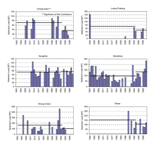
**Fig. 9.** Mean annual sediment load estimations and differences in sediment flux between pre- and post-dam periods. The horizontal lines represent the mean sediment load in pre- and post-dam periods. Chiang Saen is significant at 95% confidence level.
