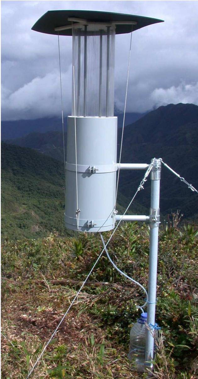
**Fig. 1.** Passive fog collector.
