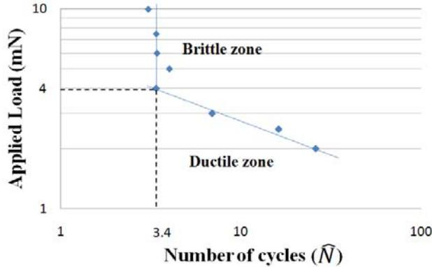
Figure 6: Wöhler diagram of the contact fatigue results
