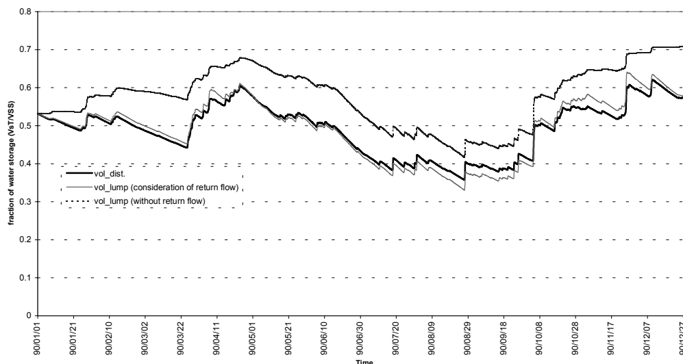
Fig. 10. Comparison of modelled soil water storage in the Upper Reno catchment. Solid line: distributed model; thin solid line: lumped model with return flow; dash line: lumped model without consideration of return flow.
