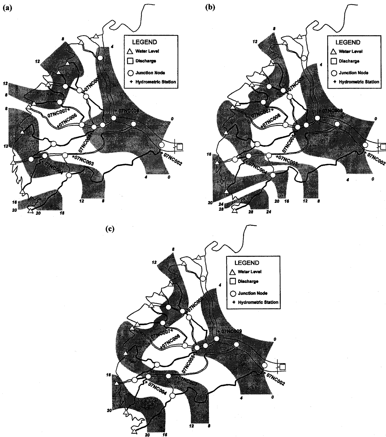
Fig. 8. (a) Four hour discharge isochrones through the Slave Delta in May 14, 1980 for an inflow of 2800 \text{ m}^3 \text{ s}^{-1} , (b) Four hour discharge isochrones through the Slave Delta in August 20, 1980 for an inflow of 3010 \text{ m}^3 \text{ s}^{-1} , (c) Four hour discharge isochrones through the Slave Delta in October 7, 1980 for an inflow of 3680 \text{ m}^3 \text{ s}^{-1} .
