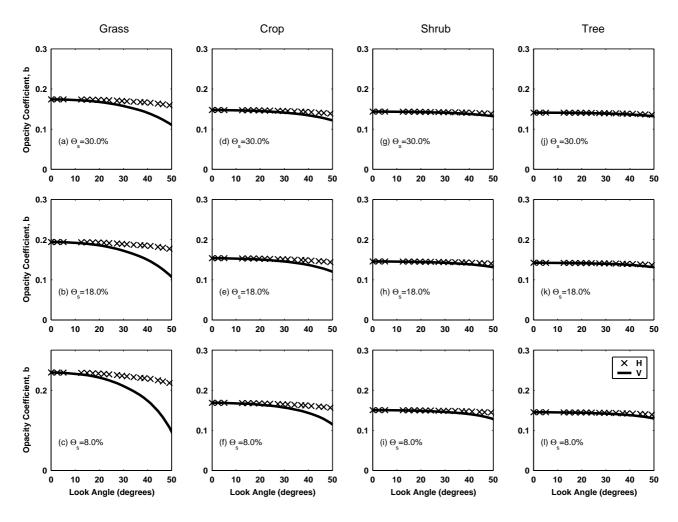
Fig. 3. The effective value of the opacity coefficient, b, required to make accurate retrievals with the two-source Fresnel model as a function of look-angle for three different soil wetness conditions and four different vegetation covers.
