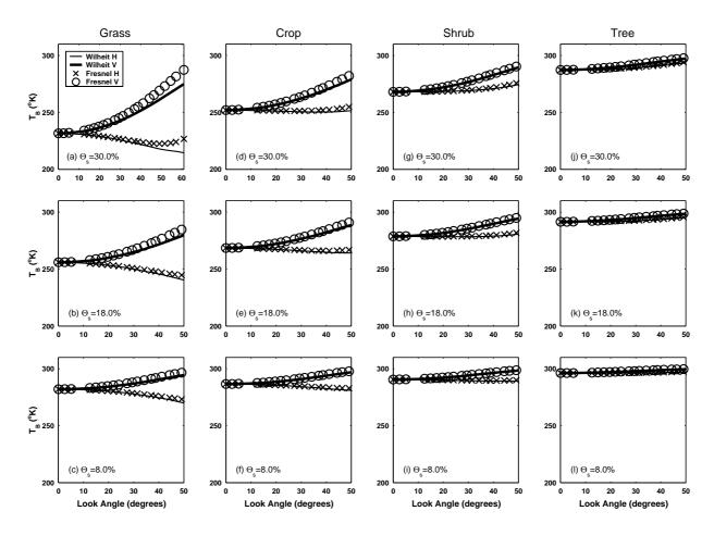
Fig. 2. Microwave brightness temperature (°K) as a function of look-angle (°) for three different conditions of soil wetness (8, 18, and 30%) and four different vegetation covers specified in Table 1 using a constant opacity coefficient, b, the value being specified to ensure equality between the two models at the nadir.
