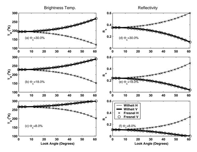
Fig. 1. Comparison of the microwave brightness temperature (°K) and soil reflectivity (no units) calculated for bare soil using the extended Wilheit (1978) model and the two-source Fresnel model for three different soil wetness conditions.
