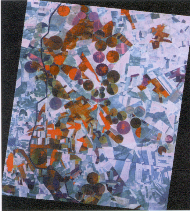
Fig. 2. Colour composite of the TMS-NS001 data (band 4,6,3). The TMS-NS001 was on board of NASA's ER2, 29 June 1991, 12.21 GMT, Barrax, Spain, 18.5m ground resolution (862 by 777 pixels or 15.9km by 14.4km, UTM coordinates at upper left corner: easting=568245.18750m, northing=4333005.0m). The circular shapes are due to pivot irrigation.
