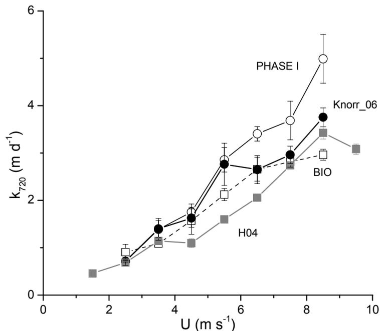
**Fig. 7.** Wind speed dependence of computed gas transfer coefficients from this work (solid black circles), the PHASE I (open circles) cruise, H04 (solid grey squares), and the BIO cruise (open squares), normalized to  $Sc=720$ . All cruises binned by wind speed. Error bars represent the standard error of the mean (if error bars are not visible they are the size of the symbol).
