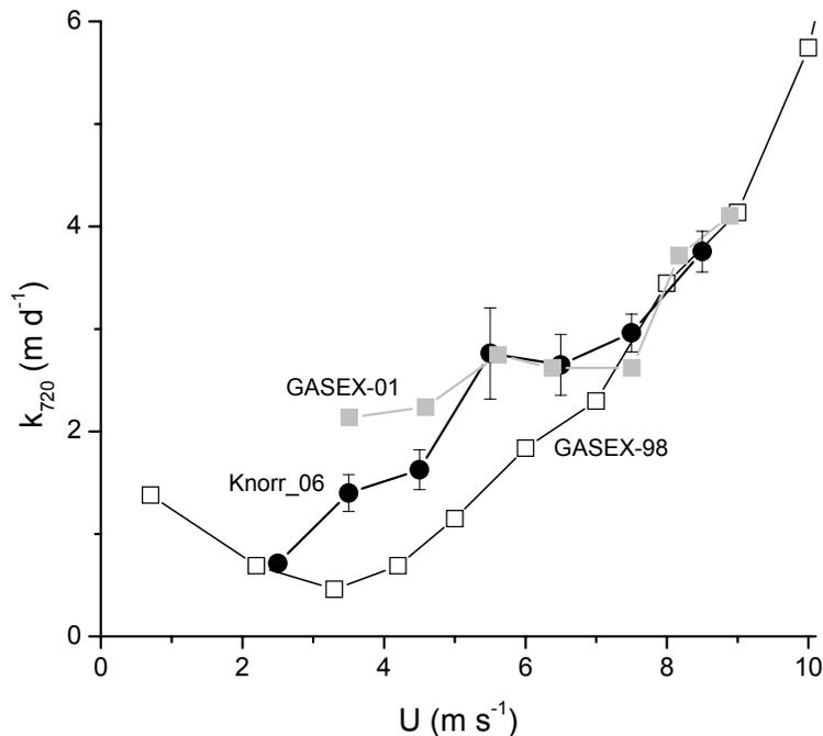
**Fig. 8.** Wind speed dependence of computed gas transfer coefficients from this work (solid black circles), the GASEX-98 (McGillis et al., 2001) cruise (open squares), and the GASEX-01 (McGillis et al., 2004) cruise (grey closed squares), normalized to  $Sc=720$ . All cruises binned by wind speed. Error bars represent  $\pm 1$  s.e.
