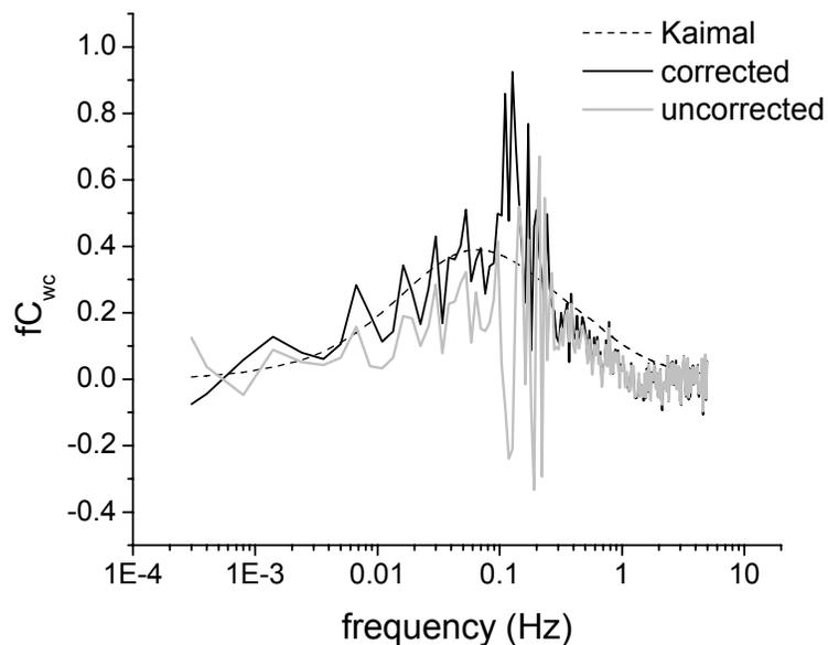
**Fig. 2.** DMS w frequency weighted cospectra from the morning of 11 January 2006. The solid black line is the cospectrum corrected for ship motion, solid grey is the motion uncorrected cospectrum, and the dashed line is the idealized scalar cospectrum from Kaimal et al. (1972).
