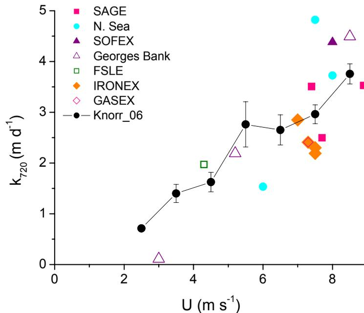
**Fig. 9.** Comparison between  $k_{720}$  for DMS measured in this study and those measured by various dual tracer experiments. The Knorr\_06 data has been binned by wind speed and error bars represent  $\pm 1$  s.e. All the data has been normalized to a  $Sc=720$ .
