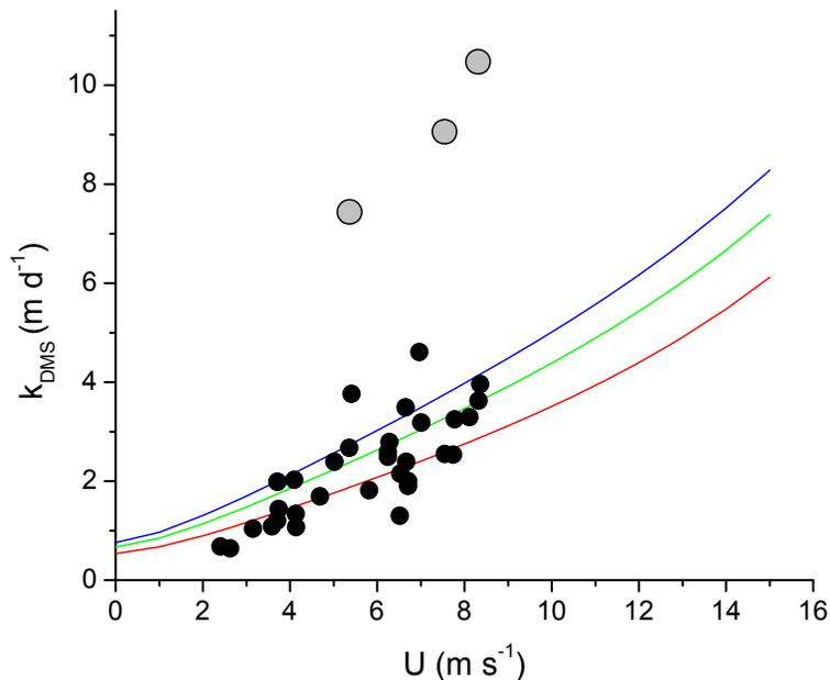
**Fig. 11.** The wind speed dependence of the DMS gas transfer coefficient measured in Knorr\_06 (closed circles) compared to various NOAA/COARE model runs with different tunable parameter  $A$  values ( $A=2.0$ , blue line;  $A=1.7$ , green line;  $A=1.3$ , red line).
