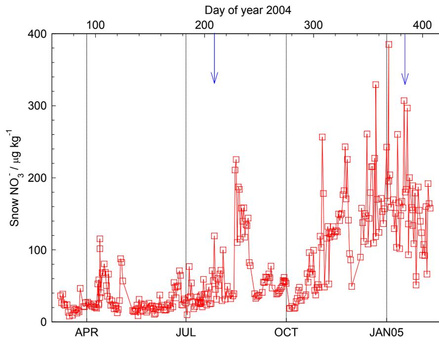
**Fig. 1.** Nitrate concentrations measured in surface snow samples collected approximately daily at Halley, Antarctica, in 2004 and early 2005. Month markers and grid lines refer to the start of the respective months. The timing of the maximum of the two largest SPE's of the period (proton flux at  $>10$  MeV more than 1000 pfu, based on NOAA Space Environment Center listing) is shown as arrows.
