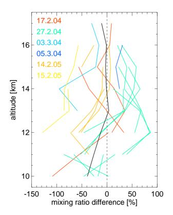
**Fig. 7.** Overview of relative differences between DIAL and ENVISAT/MIPAS from Fig. 6. The overall mean (black line) and standard deviation is  $-8.3\%\pm48.5\%$ , above  $12\,\text{km}$   $-3.2\%\pm48.8\%$ . Negative difference means DIAL more humid.
