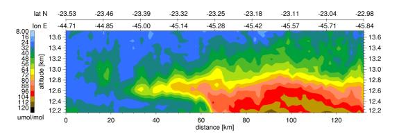
**Fig. 2.** Vertical cut of DIAL water vapor volume mixing ratio through the anvil outflow of a deep convective system into the clear-sky TTL on 3 March 2004 at 13:06 UTC. The horizontal resolution is 2 km, the vertical 100 m (300 m) at the bottom (top). The thunderstorm was located  $\sim$ 100 km to the right.
