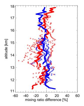
**Fig. 5.** Overview of all relative differences from Fig. 4 between DIAL and FISH (FLASH) in blue (red); overall averages solid. The average profiles have discontinuities at altitudes where individual profiles stop. Above 15.5 (17.3) km altitude the average difference with FISH (FLASH) is from Fig. 4a only. Positive difference means DIAL drier. There is no significant altitude-dependent bias.
