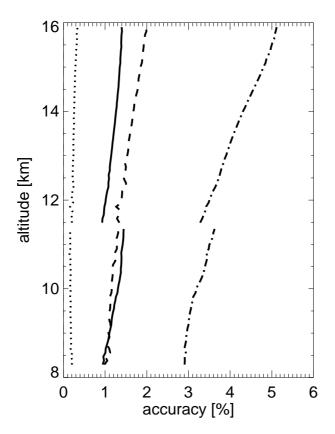
**Fig. 1.** DIAL accuracy for two profiles of Fig. 3 obtained with the strong (above 11.5 km) and medium (below) absorption lines of Table 1. Sensitivities with respect to laser spectral impurity (solid), Rayleigh Doppler effect (dash-dotted), pressure (dashed) and temperature (dotted) are plotted versus altitude. The reference parameters and their variations are listed in Table 2.
