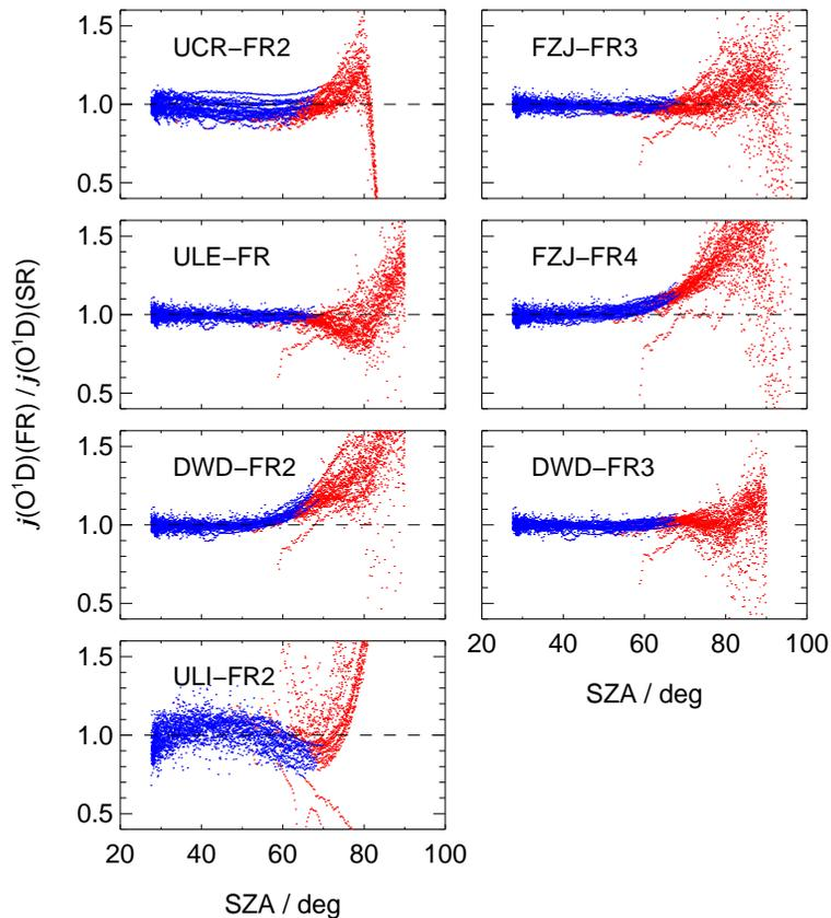
**Fig. 15.** Ratios of  $j(\text{O}^1\text{D})$  photolysis frequencies as a function of solar zenith angle during the period 1–12 June 2005. Red data points indicate values below 10% of maximum values.
