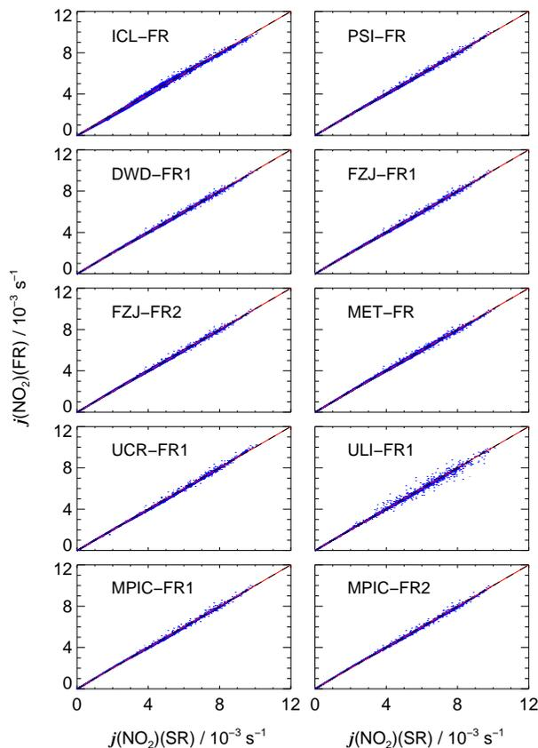
**Fig. 12.** Correlation plots of  $j(\text{NO}_2)$  photolysis frequencies from FZJ-SR1 and  $j(\text{NO}_2)$ -FR during the period 7–12 June 2005. Full lines correspond to 1:1 relationships after application of the calibration factors from Table 4.
