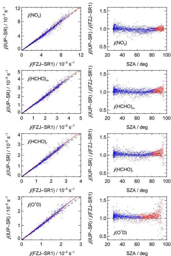
**Fig. 8.** Left: Correlation plots of photolysis frequencies from FZJ-SR1 and IUP-SR during the period 2–12 June 2005 ( $N=1693$ ). Data of FZJ-SR1 were interpolated to the measurement times of IUP-SR. See Fig. 7 for more details.
