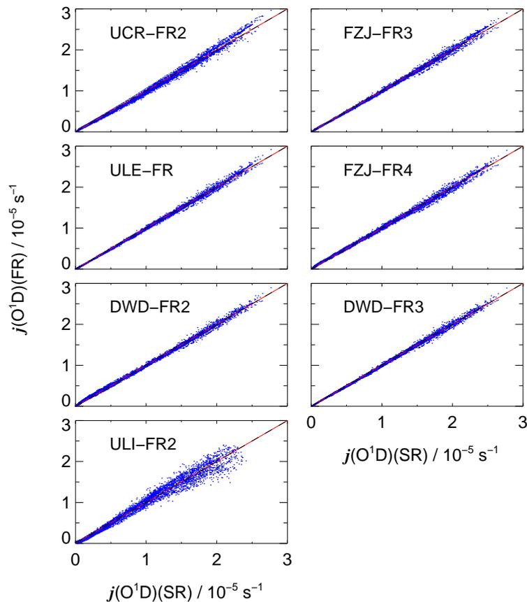
**Fig. 14.** Correlation plots of  $j(\text{O}^1\text{D})$  photolysis frequencies from FZJ-SR1 and  $j(\text{O}^1\text{D})$ -FR during the period 1–12 June 2005. Full lines correspond to 1:1 relationships after application of the scaling factors from Table 5.
