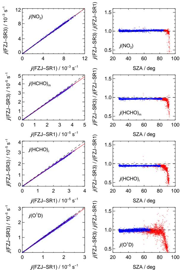
**Fig. 11.** Left: Correlation plots of photolysis frequencies from FZJ-SR1 and FZJ-SR3 during the period 1–12 June 2005 ( $N=6731$ ). Data of FZJ-SR3 were averaged over the scanning periods of FZJ-SR1. See Fig. 7 for more details.
