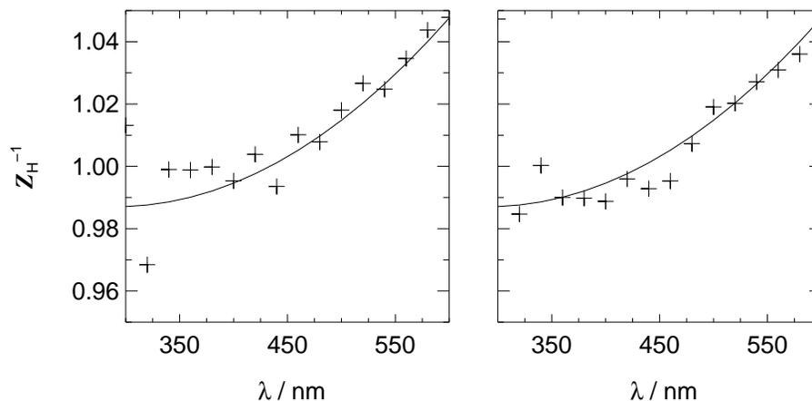
**Fig. 2.** Correction factors  $1/Z_H$  for isotropic sky radiation from the upper hemisphere as a function of wavelength. Left and right panels correspond to left and right panels in Fig. 1, respectively. Variations at short wavelengths were caused by low signals from laboratory lamps. The full lines show a fitted mean dependence considering all measured data.
