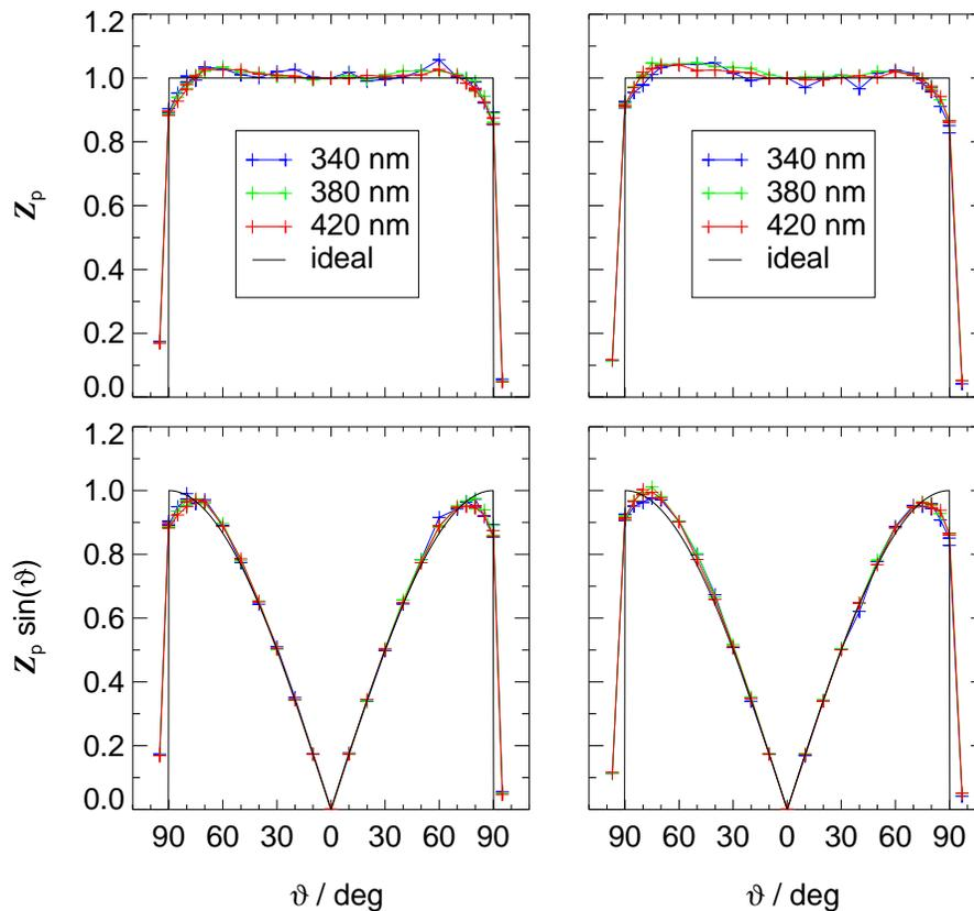
**Fig. 1.** Upper panels: Relative response  $Z_p$  of the reference instrument receiver optics as a function of polar angle and wavelength. The two plots show the dependencies for two perpendicular orientations with respect to azimuth angles. Lower panels:  $Z_p$  from the upper panels multiplied by  $\sin(\vartheta)$  indicating the relative weight for an isotropic sky radiance distribution of the upper hemisphere.
