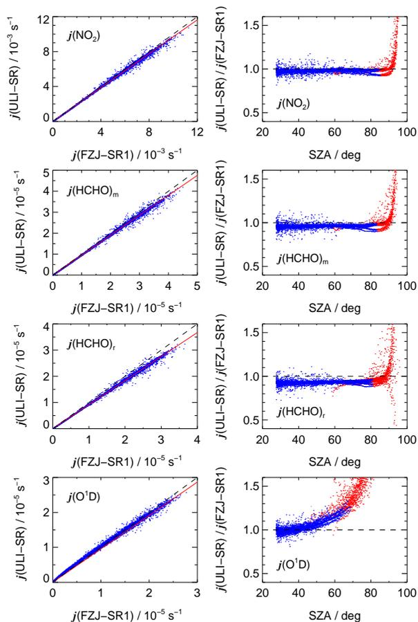
**Fig. 9.** Left: Correlation plots of photolysis frequencies from FZJ-SR1 and ULI-SR during the period 1–12 June 2005 ( $N=5960$ ). Data of ULI-SR were interpolated to the measurement times of FZJ-SR1. See Fig. 7 for more details.
