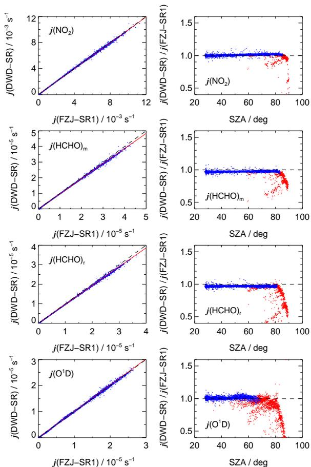
**Fig. 10.** Left: Correlation plots of photolysis frequencies from FZJ-SR1 and DWD-SR during the period 1–12 June 2005 ( $N=5975$ ). Data of DWD-SR were averaged over the scanning periods of FZJ-SR1. See Fig. 7 for more details.
