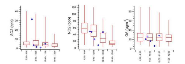
**Fig. 3.**  $SO_2$ ,  $NO_2$ , and organic carbon concentrations measured during the MCMA-2003 campaign. Whisker plots indicate the diel variability of measurements over the entire campaign. The five case studies discussed here – shown as the blue dots – easily fall within the variability seen throughout the campaign.
