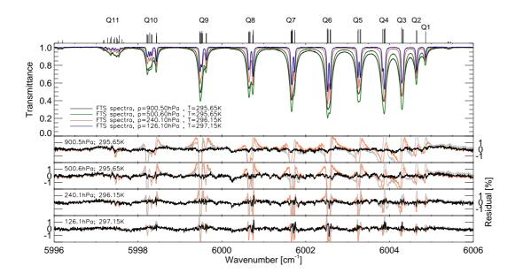
Fig. 2. Fit results of the multi-spectra inversion for the Q branch. The upper panel depicts the N<sub>2</sub> broadened FTS spectra. The lower panels show the fitting residuals for each FTS spectrum separately in black (measured-modelled times 100). The red lines indicate residuals if no changes to the HITRAN database were applied. The gray lines show residuals using the HITRAN database but replacing broadening coefficients with results by Pine (1992, 1997) in the fundamental.
