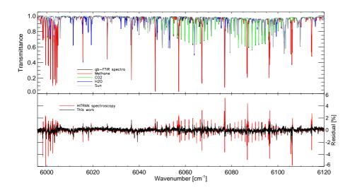
Fig. 7. Spectral fit of a ground based FTIR measurement in Bremen, Germany, measured with 45 cm optical path difference at 63.51° SZA on 3 July 2006. The upper panel shows the spectrum and the contributions of the individual gases as well as the sun. The lower panel depicts the fit residuals (Measured-modelled) for the spectroscopic parameters from this study and HITRAN, respectively.
