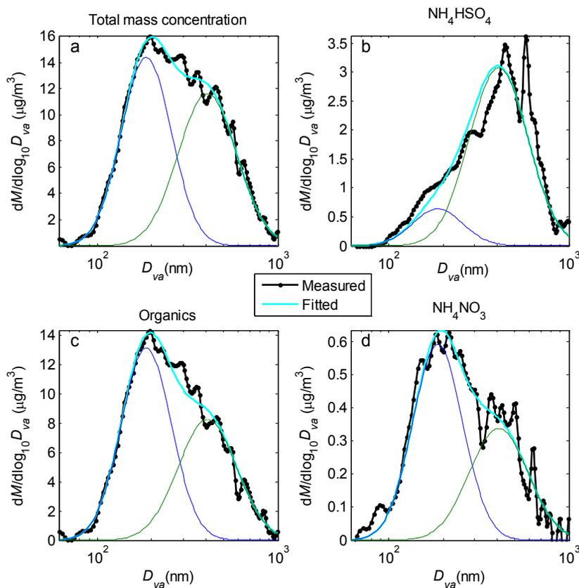
**Fig. 5.** Measured and fitted mass size distributions of total mass,  $\text{NH}_4\text{HSO}_4$ , organics, and  $\text{NH}_4\text{NO}_3$  for the aerosol observed in a thin layer above cloud on 27 July 2005. The thick black and cyan lines represent the measured and fitted mass size distributions. The thin blue and green curves are fitted mass size distributions for each lognormal mode.
