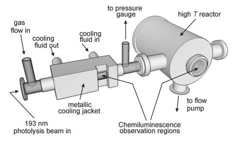
**Fig. 2.** Experimental apparatus showing the coupled low- and high-temperature reaction cells used for the determination of  $k_{\text{R1}}(T)$  and for the O(<sup>3</sup>P) yield  $k_{\text{R1c}}/k_{\text{R1}}$ .
