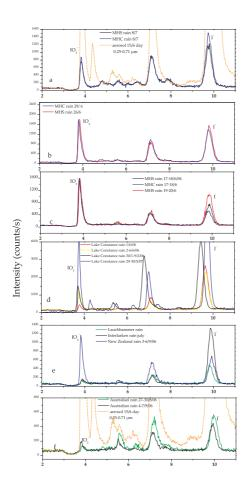
**Fig. 8.** IC-ICP-MS chromatograms of rain samples from the Southern and Northern Hemispheres. MHS is samples from Mace Head Station and MHC is samples from Mace Head Cottage. Note that in part (a) and (f) Mace Head aerosol sample  $0.25-0.71 \mu m$  from the 15/6/06 is overlaid for a comparison between aerosol and rain speciation.
